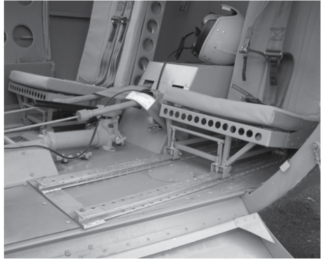
A door in the cabin bulkhead accesses the rear rooms. Both handmade seats are fore and aft adjustable with spring loaded pins. A hydraulic pump actuates the flaps.
