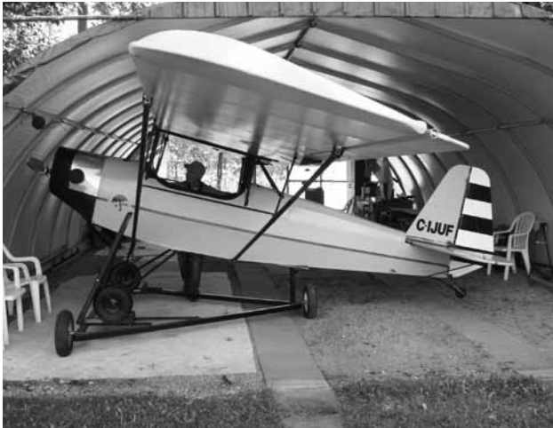
Jimmy Kennedy's hangar requires that the plane be pushed in sideways. The ramps hinge down for loading / unloading.
