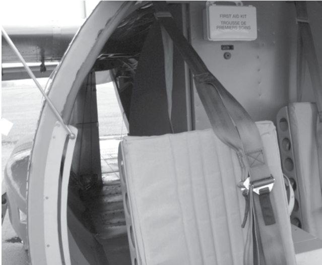
A door in the cabin bulkhead accesses the rear rooms. Both handmade seats are fore and aft adjustable with spring loaded pins. A hydraulic pump actuates the flaps.
