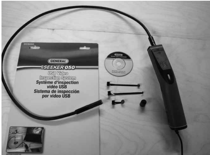
The camera includes a mirror, a hook, a magnet, and a cap, plus of course the software.
