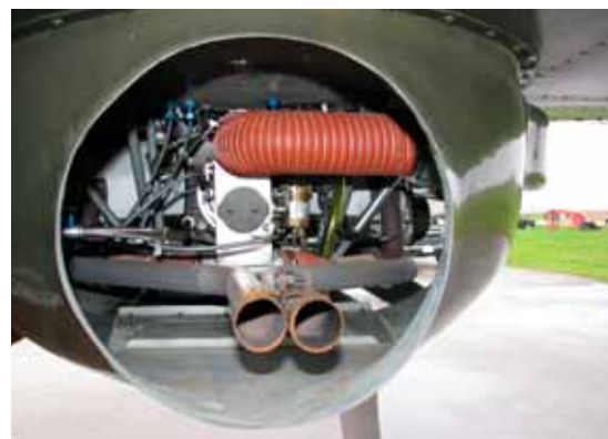
Above: How big are these pilots? It's easy to do a double-take when seeing this out of the corner of your eye. Each engine has good access via dropdown panels; and paired exhausts provide good heat for the carburetors.
