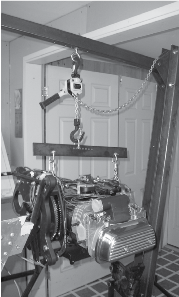
Top: some of the connecting hardware; securing the engine to the engine stand; and left, lifting the engine off the bench.
