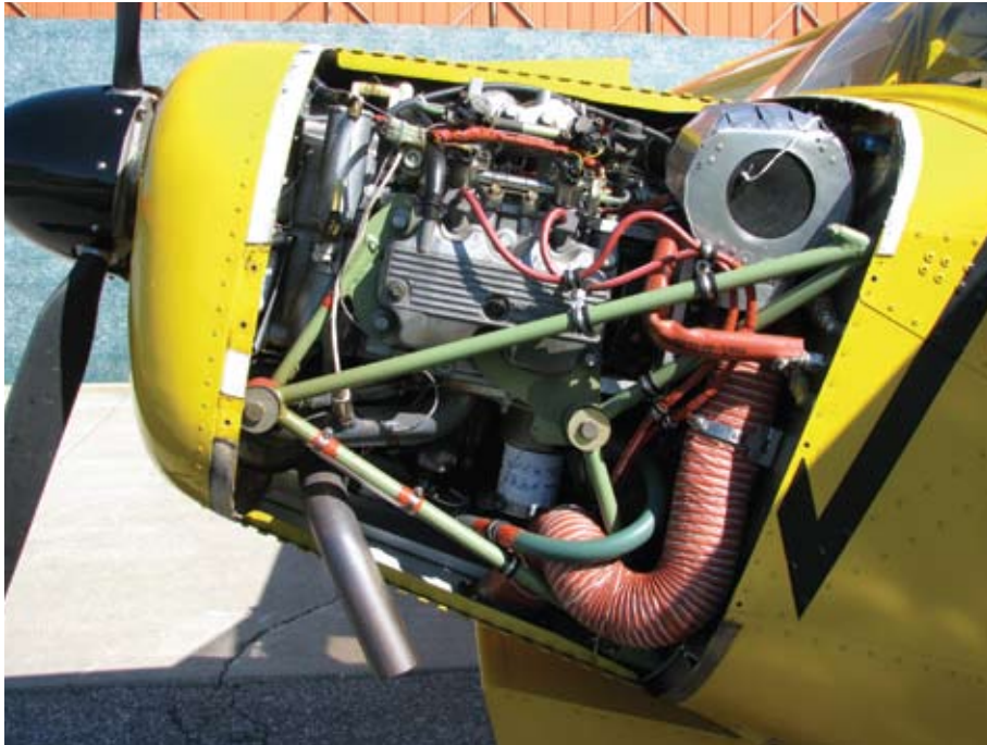
Exhaust is under the chin and has an O2 sensor for the computer. Air intake is at the firewall and has a temp monitor.
